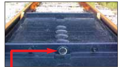
Large, 3"-diameter flow-through channels allow spills to quickly travel from one pan to the next. Channels are located at the low point in each Center and Side Track Pan.
