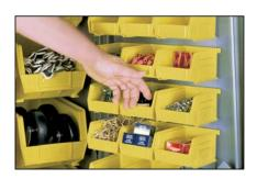
REMOVABLE PLASTIC PARTS BINS increase storage density, speed selection and retrieval. Corrosion resistant, and impervious to most solvents, Safety Yellow plastic bins easily clip on and off racks welded to cabinets and doors.
