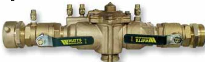
The Backflow Preventer is designed to provide protection of the safe drinking water in accordance with national plumbing codes and water utility authority requirements. They can be utilized in backflow prevention programs, including high hazard cross-connections in plumbing systems, or for containment at the service line entrance. Features two in-line, independent check valves with an intermediate relief valve. Standardly furnished with ball type test cocks.
