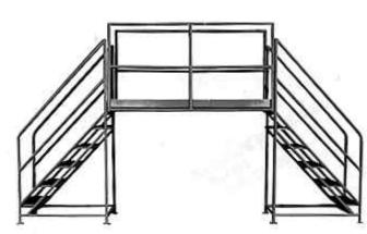
To get the most use from a minimum amount of floor space, Ballymore Crossovers provide safe, convenient access over conveyors, assembly lines, piping or other obstructions. The comfortable 48° stair slope allows worker to descend facing outward. Any combination of 6 stair heights and 5 bridge lengths is available in 3 standard widths to satisfy most requirements. Custom sizes and configurations are also available.
