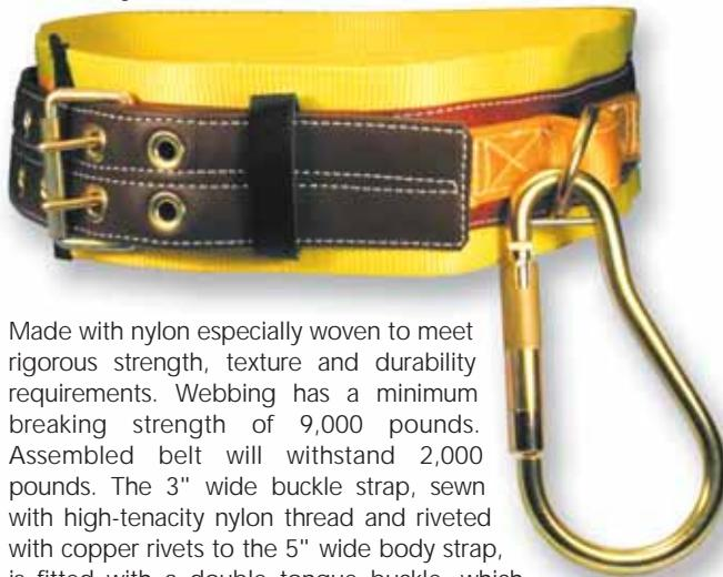
Made with nylon especially woven to meet rigorous strength, texture and durability requirements. Webbing has a minimum breaking strength of 9,000 pounds. Assembled belt will withstand 2,000 pounds. The 3" wide buckle strap, sewn with high-tenacity nylon thread and riveted with copper rivets to the 5" wide body strap, is fitted with a double tongue buckle, which enables fast engagement and release of belt. Ship. wt. 5 lbs.
