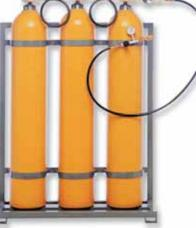
SCBA manifolds are rated up to 6000 psi. Can be installed in a station or in an apparatus if cylinders are difficult to access. Includes 6000 psi metering control valve for each bank, an inlet valve for filling the system, and a #4 male JIC on each bank inlet. Ship. wt. 8 lbs.
