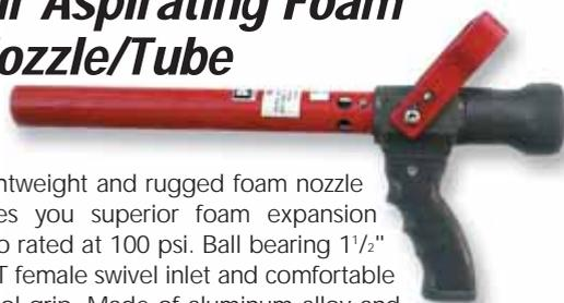
Lightweight and rugged foam nozzle gives you superior foam expansion ratio rated at 100 psi. Ball bearing 1 1/2" NST female swivel inlet and comfortable pistol grip. Made of aluminum alloy and stainless steel with powder-coated red finish. *Ship. wt. 5 lbs.*
