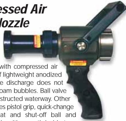
Ideal for use with compressed air foam. Made of lightweight anodized aluminum. The discharge does not "flatten out" foam bubbles. Ball valve has 1 3/8" unobstructed waterway. Other features includes pistol grip, quick-change rear valve seat and shut-off ball and smooth bore tip with smooth inside taper for solid stream. NST threads. *Ship. wt. 5 lbs.*
