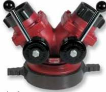
Suction Siamese is made of lightweight aluminum alloy. Used to feed pumper suctions or aerial platforms with one or two,  $2^{1}/2^{"}$  or 3" hose lines. Has self-locking valves for positive handle positioning. Available in sizes  $2^{1}/2^{"}$  to 6" female swivel x (2)  $2^{1}/2^{"}$  NST swivel female valved inlets. *Ship. wt. 19 lbs.*
