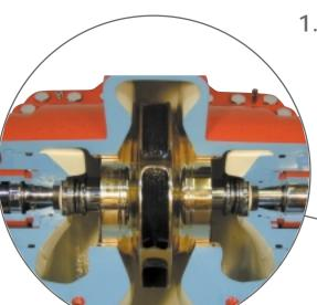
1. Internal Self-Flushing Mechanical Seals
