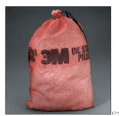
The 3M<sup>™</sup> Petroleum Sorbent Pillow T-240 is a selective sorbent which will "sorb" hydrocarbon-based liquids (oleophilic) and repel aqueous-based liquids (hydrophobic). These open mesh bags of particulate sorbent are excellent for handling large quantities of light oil in confined spaces such as sumps, catch basins, bilges, or settlement ponds. Designed for long term use, they are UV resistant and will not deteriorate or sink.
