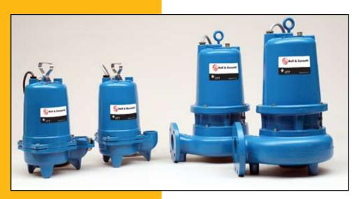
Bell & Gossett also offers a full line of submersible wastewater pumps from 11/4" discharge sump pumps to 4" discharge sewage pumps. Construction materials can be thermoplastic, stainless steel or cast iron. All pumps are rated for continuous duty. Many feature long life Silicon Carbide mechanical seal faces that set our pumps apart from the competition.
