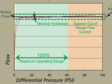
The unique features of the cartridge and unprecedented control of branch flow for any HVAC circuit can be seen in Graph 1. Even when differential pressure is increased to 1.5 times the rated operation of the cartridge flow, control is maintained.
