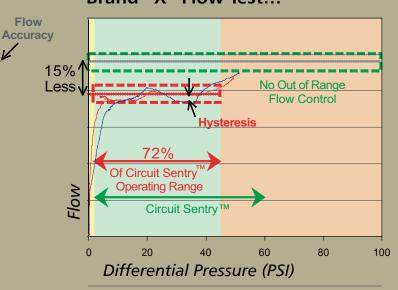
Variable-orifice cartridges aren't designed for this precise flow control and often require as many as four different spring ranges to achieve similar results for one flow.
