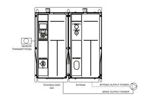
a timed sequence of events to start the pump across the line. The pump shall run at constant speed with motor overload and ground fault protection. Bypass mode will be indicated on the drive keypad. In the event of a system differential pressure failure due to a pump or motor fault, the pump logic controller shall automatically initiate a timed sequence of operation to shut the system down. In the event of an overload fault while in the "BYPASS" mode, the pump shall be locked out of operation.
