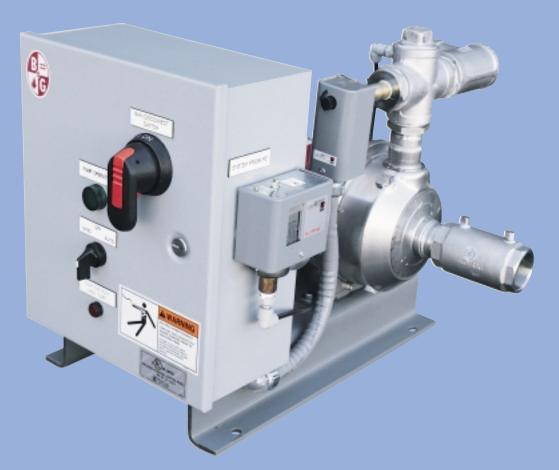
Specifically designed as a compact, easy to install and maintain package for applications where sufficient main pressure is not available or elevation is a problem. Typical installations include residences, apartment buildings, condominiums and light commercial applications. The MiniBooster is available in both one and two pump packages. Simplex capacities are from 20 to 110 GPM at a boost of 20 to 55 psig. Duplex capacities are up to 220 GPM.
