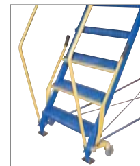
Push handle forward to gain access to ladder. Casters are raised from floor and unit becomes stationary.
