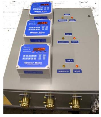
**Definition.** A triplex system has three demand regenerated mineral vessels with separate meters and controllers. Each unit regenerates when its demand set point is reached and returns to service immediately after regeneration. Two vessels are always in service providing a continuous stream of softened water.
