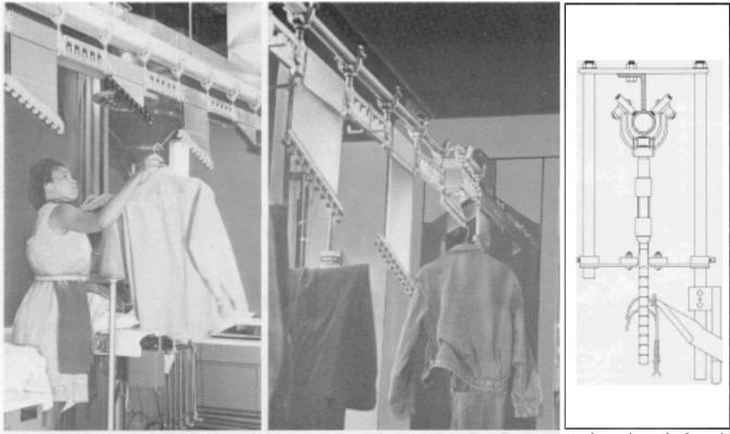
Hangers are placed on selected hooks, which correspond to discharge stations. Traveling perpeitems are discharged by passing a mechanical probe...it is that simple!
