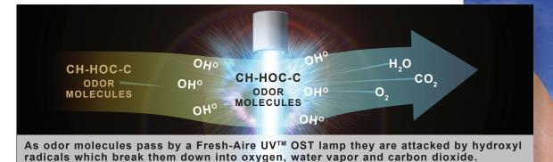
This process is known as Advanced Oxidation and is used very extensively in water treatment and clean room applications. In addition, the FDA has approved this process as an antimicrobial treatment method for food processing applications and has given it a GRAS status.
