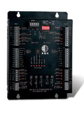
The RC-2 Reader Controller is part of the Axiom line of access control products from RBH. Its versatile design features take care of present and future needs with ease and efficiency.
