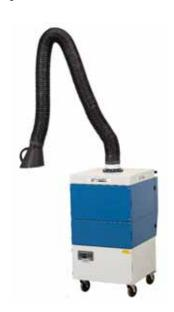
Simply swing open the air plenum access door and the inside of the cartridge filter is accessible. For cleaning, use shop air - with an air wand. The cleaning procedure requires no pulse valves or electrical components, thus preventing needless failures. The unit is supplied with a filter monitor light.
