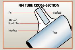
Cain Industries' patented bonding process metallurgically joins stainless steel fins to aluminum tubes for the highest heat transfer efficiency possible. Even when magnified 100x, no voids are revealed in the metallurgical bond. That is your assurance of maximum heat transfer efficiency, and a technological advantage over other types of finned tubing.
