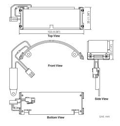
Installing this Heater Unit in the applicable dome camera allows the camera to be used in location exposed to extremely low ambient temperature.
