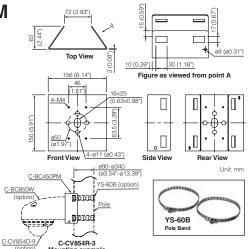
• Designed to mount TOA CCTV Cameras on a pole in conjunction with the optional C-BC850W and YS-60B.
