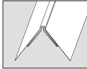
*Smooth exposed metal has minimal bond to mud. Only the short paper tabs hold the bead on the wall.*
