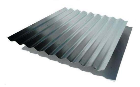
Roofing Sheets – galvanized steel corrugated roofing sheets. Used for domestic and commercial applications. Once installed this sheets has a net coverage of 24" width. It can be produce up to 22' long in 24ga and 26ga.
