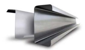
Purlins – "C" and "Z" shape beams made of hot dipped galvanized steel, conforming to ASTM Designation A446 Grade 50, for Structural Quality Steel with a minimum yield strength of 50,000 p.s.i. and G-90 galvanized coating. Sizes available from 4" to 10" high and from 2  $\frac{1}{2}$ " to 3  $\frac{1}{2}$ " width.
