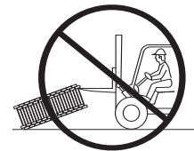
DO NOT lift Wood I Beam joists by top flange.
