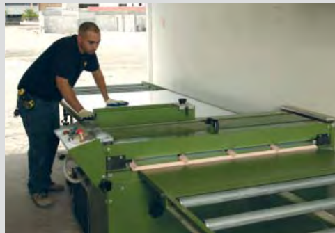
Middle: The Knauf KoolDuct V-Groove Table simplifies fabricating ductwork on-site.
