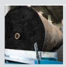
The encapsulant edge coating eliminates airstream flaring.
