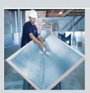
The fully sealed duct seams combined with our patented jointing system produces ductwork with minimal leakage, meeting SMACNA's Leakage Class 6.
