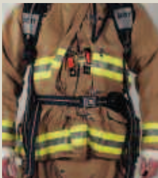
Photo 2 – The upper chest harness strap closes with a bayonet clip that is engaged as the coat is closed. The bayonet clip is a quick, easy, yet secure closure. The storm flap then covers the clip as the first photo shows.
