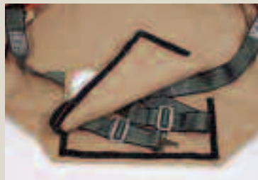
Photo 4 – When the flap is pulled, the lower torso portion of the harness is free to fall loose.
