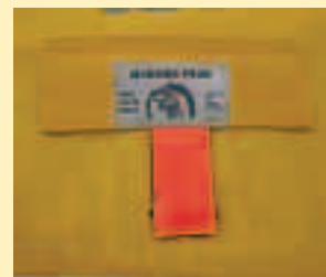
DRD Not Deployed, Flap Closed
