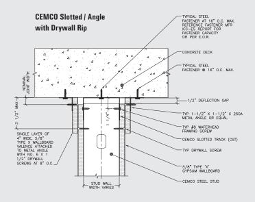
CST Combined with Various Fire Stop Materials Provides a variety of Detailed Assembly Options
