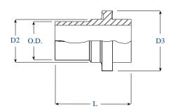
The MJ Adapter Kit consist of: HDPE MJ Adapter with metal insert, Metal Gland, Gasket, and attachment Bolts and Nuts.
