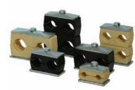
Twin Series Pipe Clamps Range: 0.25 in. (6.4 mm) through 1.66 in. (42 mm) Pressure: 1,500 psi maximum Material: Zinc Plated, 304SS, 316SS, Plain Carbon Steel Clamp Halves: Polypropylene, Santoprene
