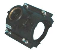
An electrofusion saddle is an excellent way to connect threaded valves to ISCO HDPE pipe. The saddle requires a small number of tools to install. Saddles are available with a female threaded outlet 3/4"- 2" sizes. Tools needed to install the saddle are the electrofusion processor, hole cutter, and manufacturers' clamping assembly (when not integral with the saddle).
