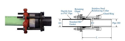
Kit Contains: -HDPE Bell MJ Fitting with stainless, reinforced support ring -Ductile iron, C110, heavy body gland ring -Gasket -Special Extra Long T-bolts -Mechanical Joint Restraint for PVC Note: Also available for connecting to Ductile Iron pipe.
