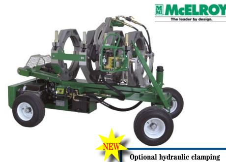
The No.618 is a self contained or electric hydraulic fusion machine. The No.618 allows for butt fusion of most fittings without special holders or removal of outer jaw. The carriage can be easily removed from the chassis for in-ditch use. A built-in hydraulic pipe lift aids in the handling of pipe. It incorporates McElroy's Patented Centerline Guidance System and is DataLogger ™compatible.
