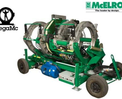
The No.1236 MegaMc is an electric hydraulic fusion machine. The machine allows for butt fusion of most fittings without special holders or removal of the outer jaw. McElroy's unique semi–automatic control system requires only one operator. Hydraulic power assists all fusion functions including the complete operation of the jaws, pipe lifts, heater, and facer. It incorporates McElroy's Patented Centerline Guidance System and is DataLogger<sup>™</sup> compatible.
