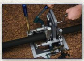
Butt Fusion – ISCO sells, rents and refurbishes equipment ideal for the job, such as the #14 McElroy Pitbull, the #2LC McElroy machine, as well as other McElroy units.
