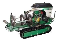
The TracStar<sup>®</sup> No.28 is a self-contained, self-propelled, all-terrain hydraulic fusion machine. The machine allows for butt fusion of most fittings without special holders or removal of the outer jaw. It fits in a standard long box truck bed for easy transport. The carriage may be easily removed for in-ditch use.
