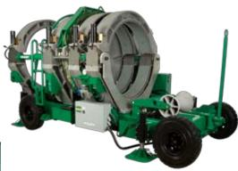
The No.2065 & 1600 MegaMc's are electric hydraulic fusion machines. The machines allow for the butt fusion of most fittings without special holders. McElroy's unique semi—automatic control system requires only one operator. Hydraulic power assists all fusion functions including the complete operation of the jaws, pipe lifts, heater, and facer. It incorporates McElroy's Patented Centerline Guidance System and is DataLogger ™ compatible.
