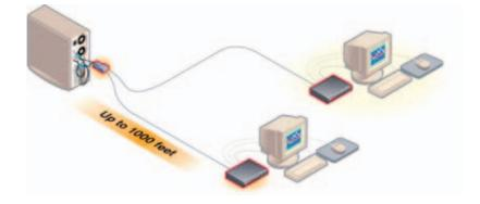
The LV1000 extender is a point-to-point KVM, audio and serial device extender up to 1000 feet. The system is a transmitter/receiver design with an interconnecting UTP cable. The skew compensation feature supports any combination of UTP cable in the extension path as well as patch panel interfaces. If the connection path is altered in any way during operation, the LV1000 will automatically adjust without any manual adjustment or user intervention.
