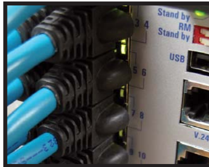
Hirschmann Industrial Ethernet Compact OpenRail Switch with RJ45 Industrial Ethernet connectors and stranded (Bonded-Pairs) TPE jacket.
