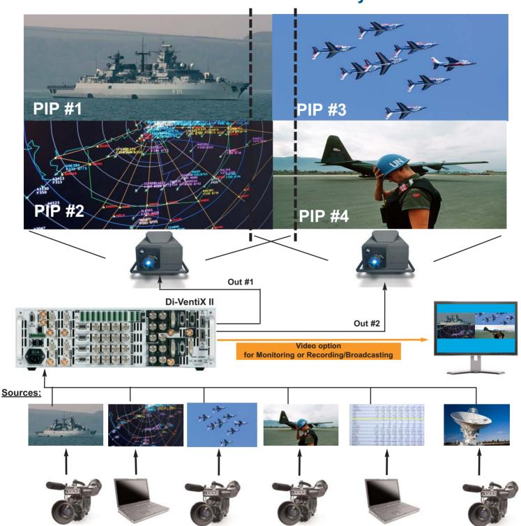
The **Di-VentiX II** is capable of displaying up to 4 live sources in Embedded Soft Edge mode, regardless of the size or position of the layer. By using a stored background, stored logos, you can achieve up to 7 layers on the screen at one time.
