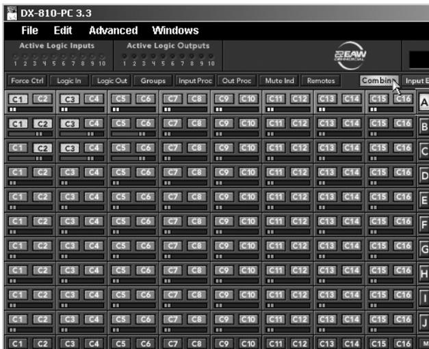
Room combining allows multiple outputs to be combined to output a single mix. Up to sixteen user-configurable combinations are available, which can be selected by remote control or a logic input
