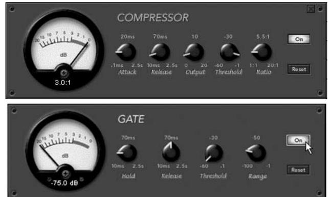
A full-featured compressor is provided for each input and output, and a full-featured gate is provided for each input
