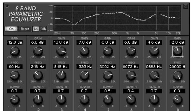
The Parametric EQ view includes five bands of control for each output, as well as a display window that graphically represents the parameter settings
