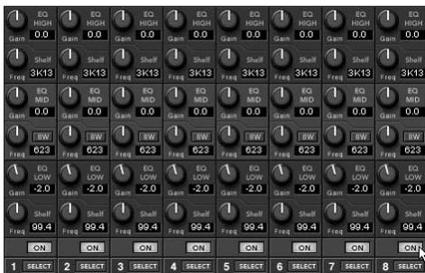
The input EQ view offers three filters for each input, with rotary gain and frequency controls for the High and Low Shelving filters, and gain, frequency, and bandwidth controls for the Bandpass filter
