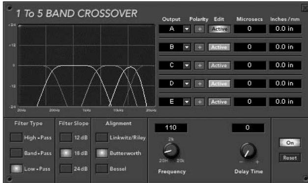
The X-over view allows grouping two or more outputs into crossover groups, with adjustable parameters including time delay, center frequency, bandwidth, three filter types, three filter slopes, and the choice of Linkwitz-Riley, Butterworth, and Bessel filter characteristics
