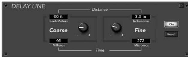
The Delay screen provides coarse and fine time delay in milliseconds and microseconds for each of the ten outputs
