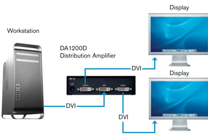
*The Emerge DA1200D DVI-D distribution amplifier provides transparent distribution of signals to two display devices using DVI cables. Fully HDCP compliant, the distribution amplifier inhibits the unauthorized distribution of digital video material through copying.*
