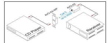
**Example System:** An AVO-A2-WP balun and AVO-A2 balun connect a remote CD player to a receiver. The distance between these devices may be up to 2,500 feet. Two patch cords with RCA connectors are required to connect the baluns to the source and destination devices.
