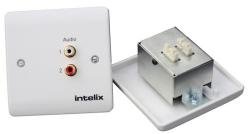
The Intelix AVO-A2-WP110-UK wallplate balun transmits two mono or one stereo analog audio signal over standard unshielded twisted pair cabling, such as Cat 5 or Cat 6. Used in pairs or with a compatible Intelix balun, the AVO-A2-WP110-UK transmits analog audio in either direction up to 2,500 feet and is ideal for corporate A/V, churches, schools, auditoriums, and almost any other situation involving audio distribution.
