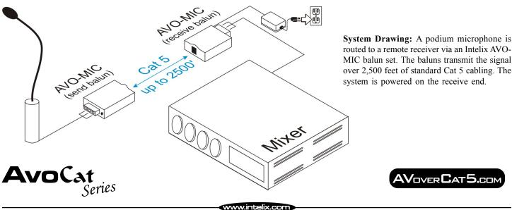
routed to a remote receiver via an Intelix AVO-MIC balun set. The baluns transmit the signal over 2,500 feet of standard Cat 5 cabling. The system is powered on the receive end.
