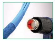
Gently apply heat from a heat gun, hair dryer or torch with an appropriate attachment. Keep the heat source far enough away so that hot metal or direct flame don't come in contact with the tubing, wires or sleeving. Move the heat around the bundle to prevent damaging the sleeving and to ensure that all areas of the tubing have been shrunk. Once cooled, your installation is complete.
