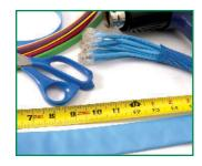
Measure the heatshrink tubing to length and cut with a scissor. The thickness of your bundle, as well as the desired final appearance, will determine the length of the tubing you cut. Generally, a piece 1 1/2" - 2" long will accommodate almost any need (such as this bundle of 10 CAT-5 network cables). Single wires, or smaller bundles, require shorter pieces.
