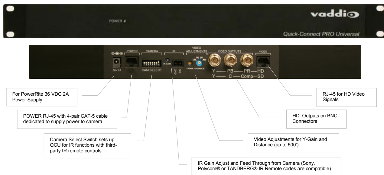
Figure 2: Quick-Connect PRO (QCP) Universal interface front panel and rear panel images with functional callouts.
