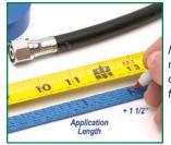
Measure the sleeving and mark the measurement with a pen or marker. Add an additional 1 1/2 - 2 inches and cut the extended length of sleeving.
