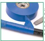
Starting at the line, take a few tight turns of tape down the application so that it covers the sleeving and extends about 1 1/2 " on the application. Make sure the tape is smooth and tight. Cut the end and press down for a smooth finish.
